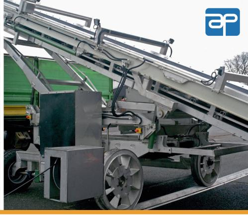
Apullma stainless steel conveyor belt cart for wagon unloading travels on V-rail
